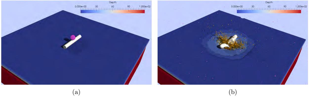
Figure II.7: Here the explosive is spherical. Again, the eventual crack pattern in (b) leads to its dismissal. Video in <https://www.dropbox.com/sh/mve31ivw15tz0nx/AAAKMaXCqp0x-GaKEAYZ2g0Pa?dl=0&preview=BlastSEC4-HD.mp4> .
