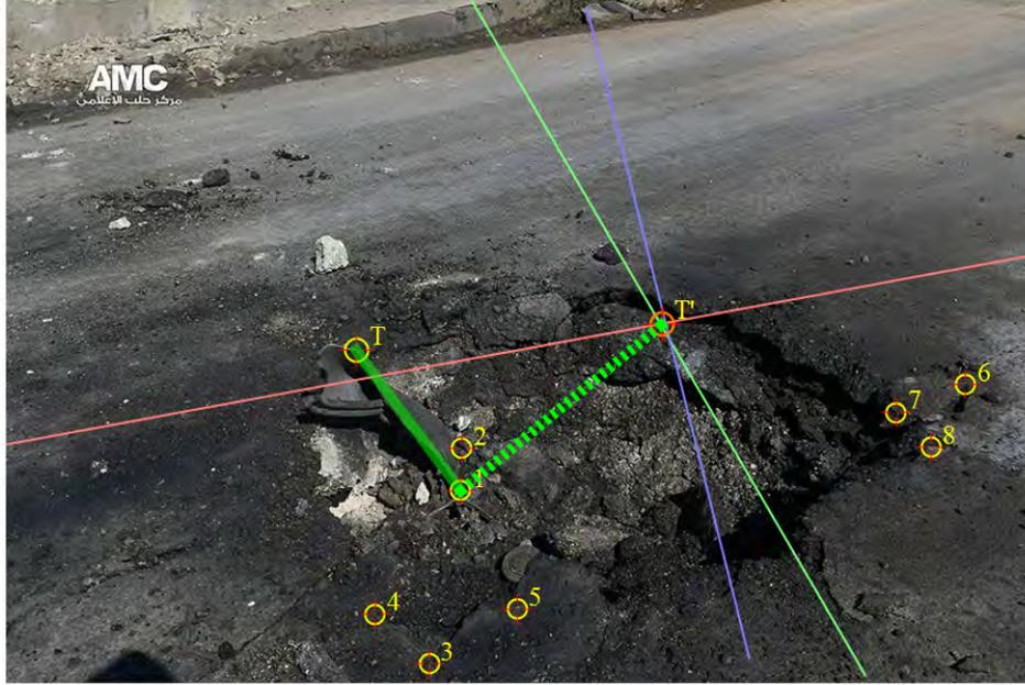
Figure I.2: The scene in image (A1) with epipolar lines showing re-projection of the tip of the (T) from the images of Group (B) into the image (A1), red, green and blue lines for (B1), (B2), and (B3) images, respectively. Red circle at their intersection shows the tip from Group (B) as it would be seen in image (A1), as a point (T'). Bold green line connects points (1) and (T) and shows direction of the pipe in Group (A), while the dashed line does in Group (B).
