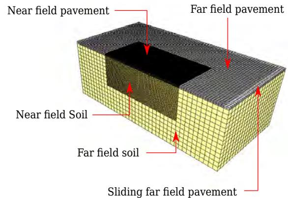
Figure II.2: Section of paved ground model.
