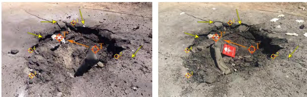
Figure 2.1: Comparison of the images (A4) (left panel) and (B2) (right panel). The observed differences in the crater shape are marked by yellow arrows. The orange arrow shows the bending direction of the pipe in image (B2). To make the comparison easier, the perspective of the image (A4) was slightly distorted (by approximately 10%) in order to make locations of four points (1–4) on the border of the crater exactly match in two images.
