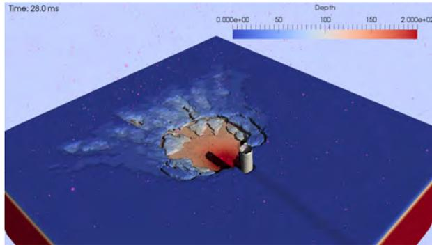
Figure 3.3: A snapshot of a 122 mm artillery rocket upon impact and explosion. This rocket is computed by using the same physical parameters as in Table 1, except that it does not have manufacturing defects. One sees no crack on the rocket casing. For dynamic visualization, see the video in <https://www.dropbox.com/sh/mve31ivwl5tz0nx/AAAKMaXCqp0x-GaKEAYZ2g0Pa?dl=0&preview=BlastSR2-J6A-HD.mp4>.
