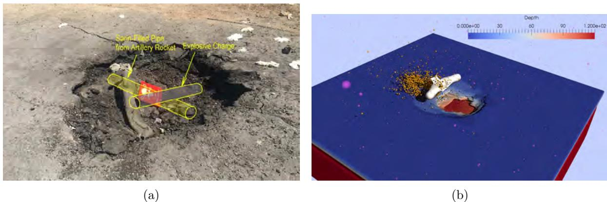
Figure II.5: (a) A possible configuration first proposed by Postol [6]; (b) A snapshot where one can see a totally different fracture pattern of the pipe. Thus, this configuration has been disproved. Video in <https://www.dropbox.com/sh/mve31ivw15tz0nx/AAAKMaXCqp0x-GaKEAYZ2g0Pa?dl=0&preview=BlastSEC2-HD.mp4>.
