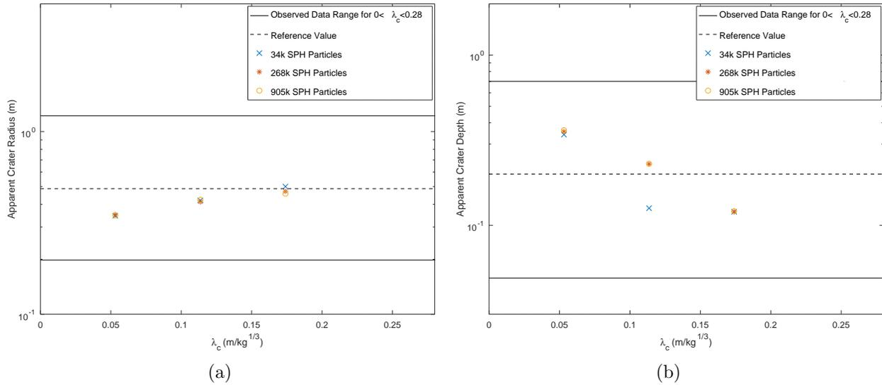
Figure II.4: Ball-shaped, 5 lb TNT charge detonated at various locations above the soil. Comparison of (a) apparent crater radius, and (b) apparent crater depth with [12].
