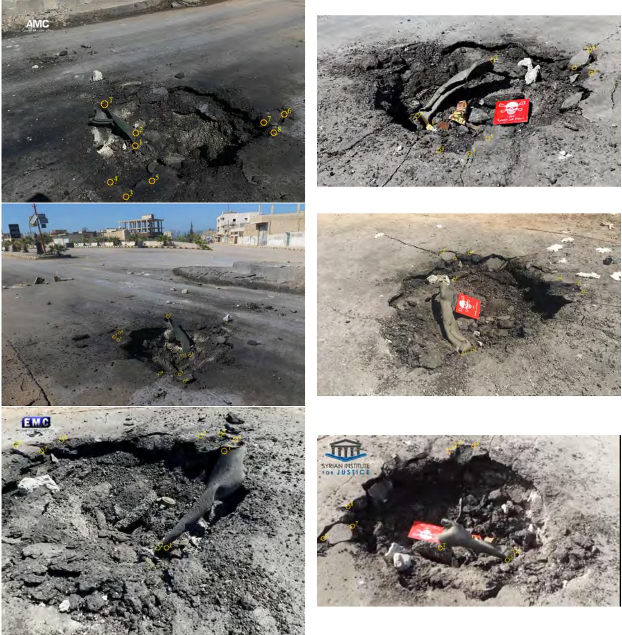
Figure I.1: Eight corresponding points (1–8) in images (A1), (B1), (A2), (B2), (A3), and (B3). The point (T) marks the tip of the pipe.
