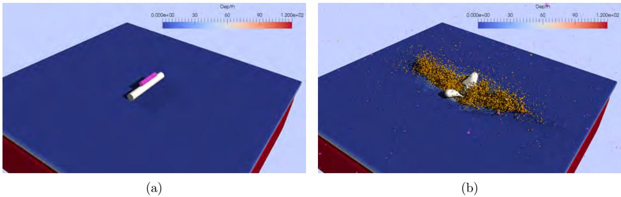
Figure II.6: This layout between the explosive (on top) and the pipe is different from that in Figure II.5. However, the fracture pattern of the pipe is similar, which is different from the pipe on the crater site so it is again dismissed. Video in <https://www.dropbox.com/sh/mve31ivw15tz0nx/AAAKMaXCqp0x-GaKEAYZ2g0Pa?dl=0&preview=BlastSEC3-HD.mp4> .
